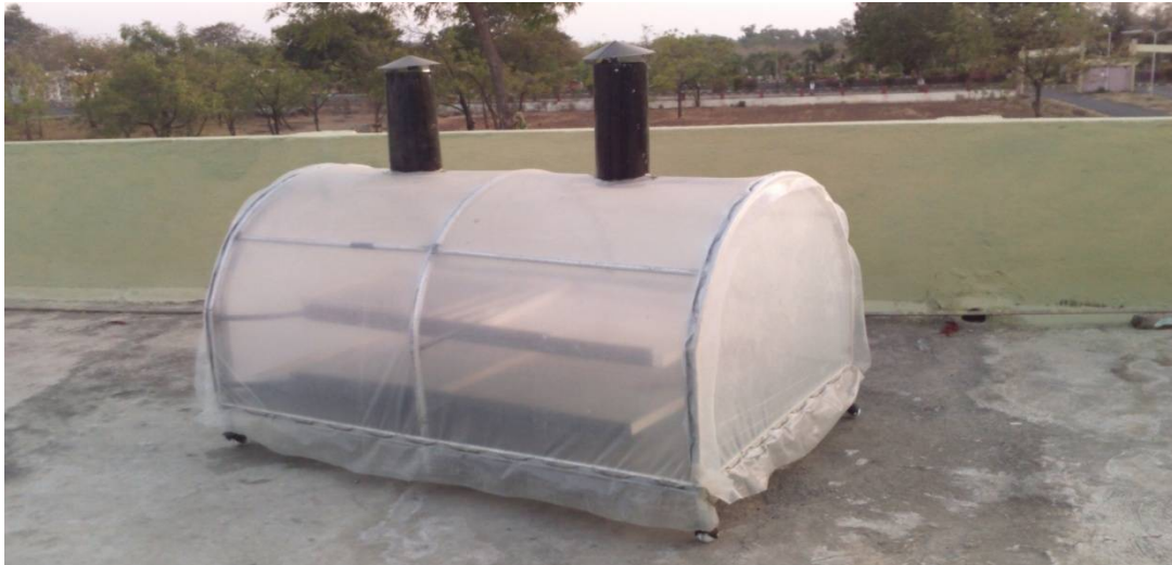
Fig.1. Mini Solar Tunnel Dryer used for experimentation
